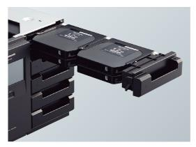
Data Archiver Magazines can be replaced easily in units of Drawers. In the event of an emergency, data can be taken out and physically transferred by the Magazine and stored at room temperature, which is useful for BCPs.
