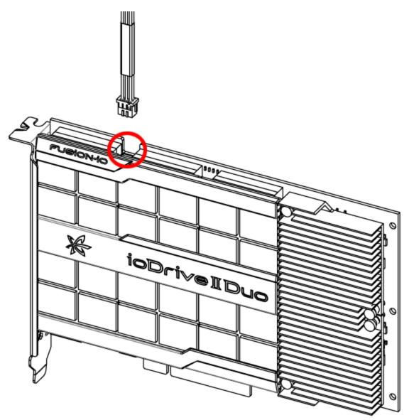
Plug the product end of the cable (shown above) into the device. Plug the other end of the cable (shown below) into an available power source cable. Consult your server documentation for available power options. Some servers may require alternative power sources and adapters to connect with the cable.
