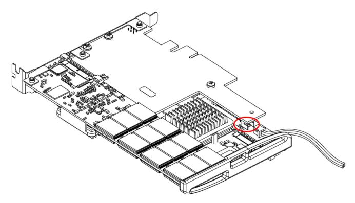
Plug the product end of the cable (shown above) into the device. Plug the other end of the cable (shown below) into an available power source cable. Consult your server documentation for available power options. Some servers may require alternative power sources and adapters to connect with the cable.
