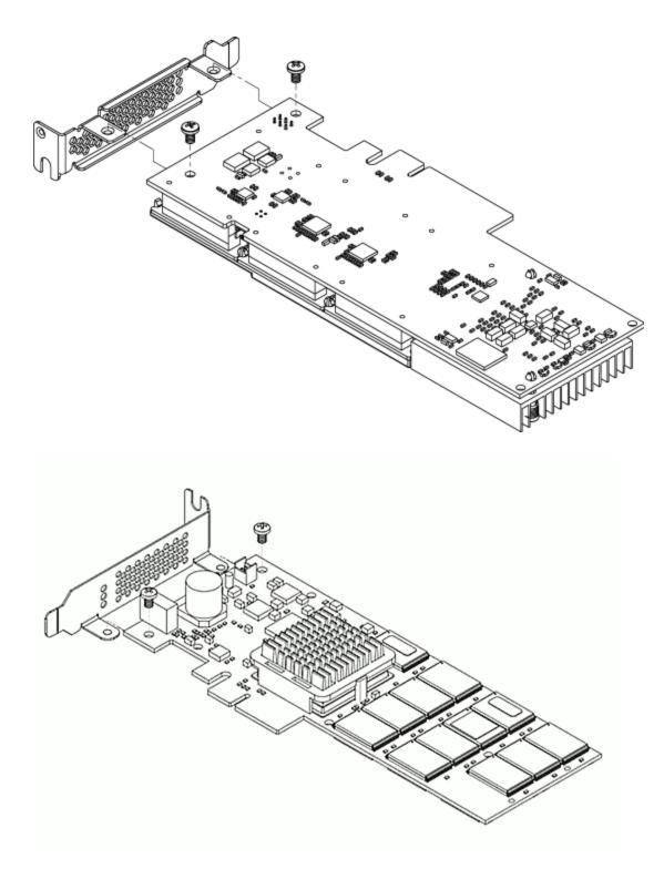
5. Attach the half-height bracket using a Phillips #1 tip screwdriver to tighten the two screws.
